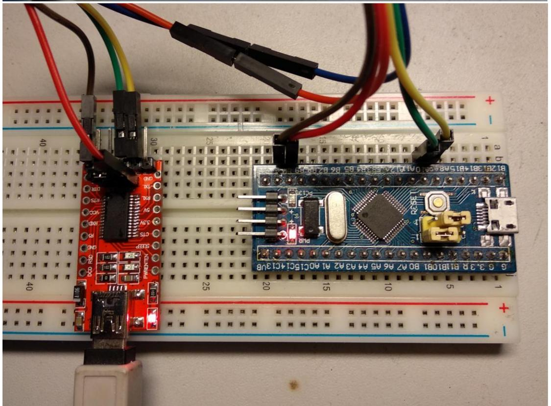
The only hardware thing left is to connect converter to PC via the micro USB cable. However, before you need to download as well as the programmer software.
