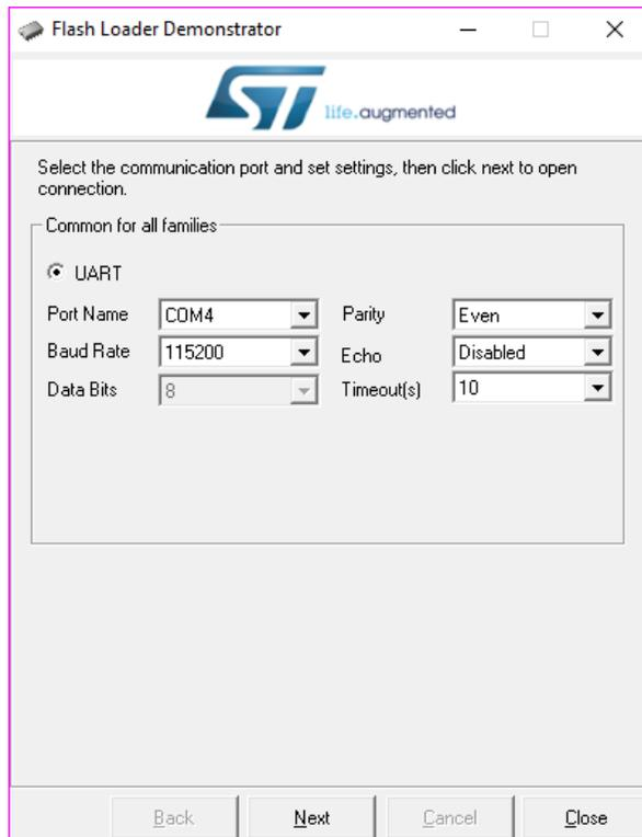
Select port, to which you connected USB-COM converter and Baud Rate 115200. (how to find out the port name see below in the attachment)
