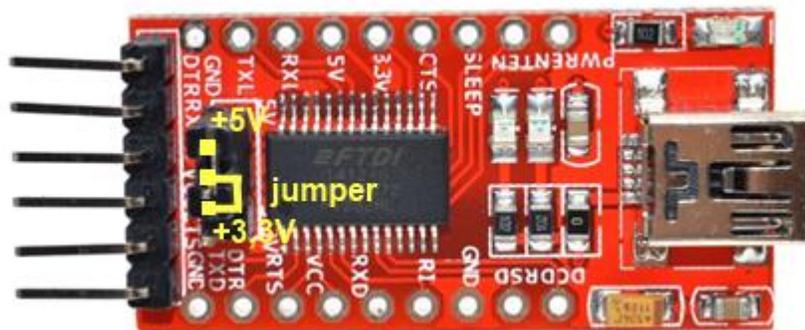
Connect the freed 5V contact with the 5V contact of the controller board contact via the red wire;
